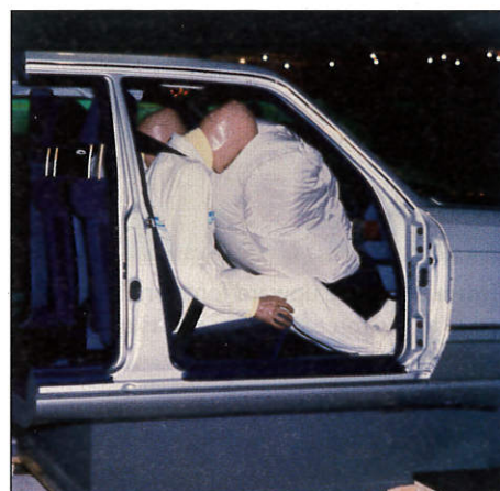
Figure 2.38 The car was originally travelling at high speed. When it hits the wall the car stops but the passenger stays in the original high speed state of motion. This results in the crash dummy hitting the steering wheel and the windshield (which is why it is a good idea to have safety belts and air bags).
