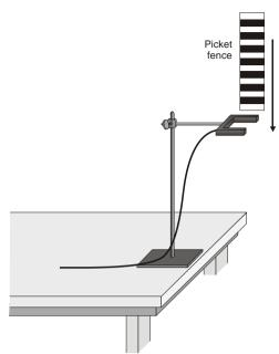
Picket Fence passes through the Photogate, the computer will measure the time from the leading edge of one bar blocking the beam until the leading edge of the next bar blocks the beam. This timing continues as all eight bars pass through the Photogate. From these measured times, the program will calculate the velocities and accelerations for this motion and graphs will be plotted.
